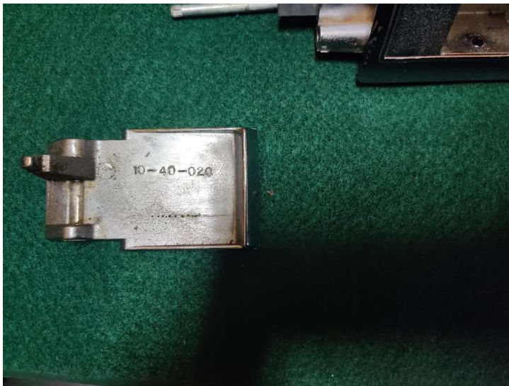
Once the pin is out far enough the external handle drops out
