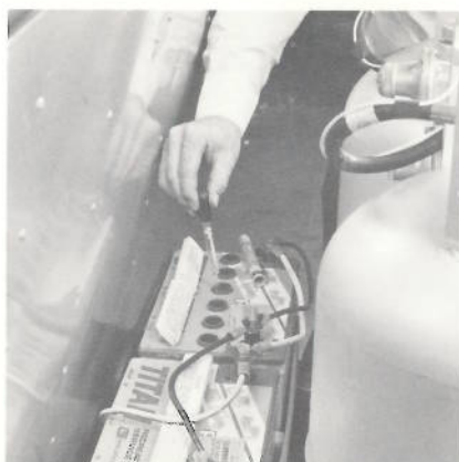
Battery Hydrometer Check
