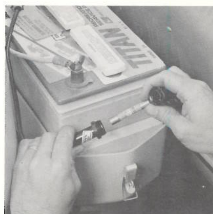
Battery In-Line Fuse
