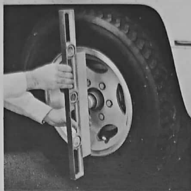
Camber Adjustment Check
