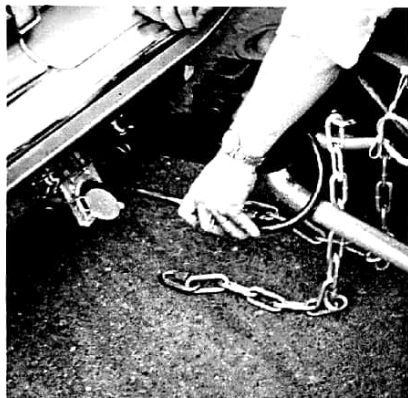
6. Hook up electrical connector
