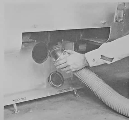
Sewer Hose Connection (Dumping)
